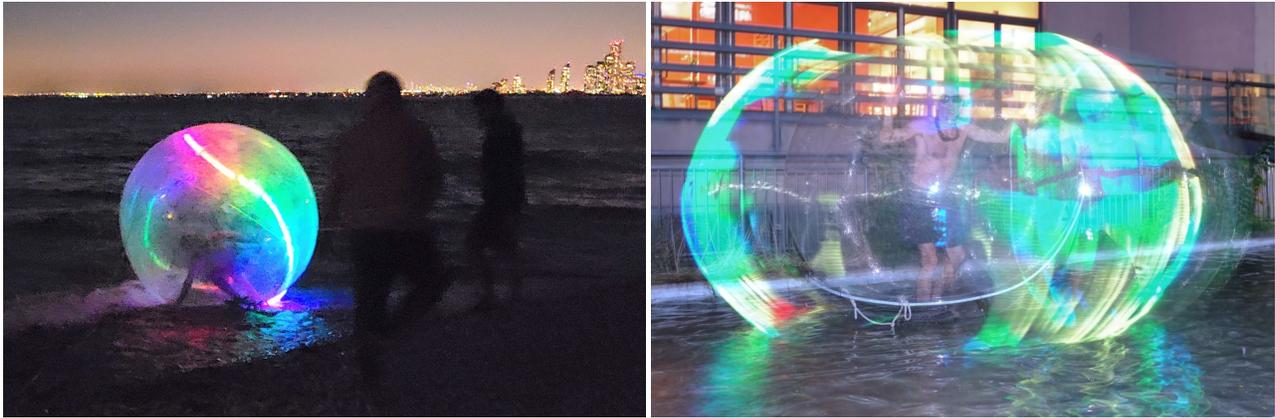
**Figure 6: Leftmost: SWIM (Sequential Wave Imprinting Machine) display is mounted in clear tubing attached to the outside of the ball to provide real-time 3-dimensional volumetric game display to the occupant of the ball as well as others observing from outside the ball. Seen at Ontario Place. Rightmost: The same setup seen in action at a fountain within the city.**
